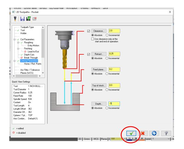
After you hit OK, you should see masterCAM draw the toolpaths. The blue lines represent the center of the cutter when it is cutting material, and the yellow lines represent the center of the cutter when it moves between geometry.
